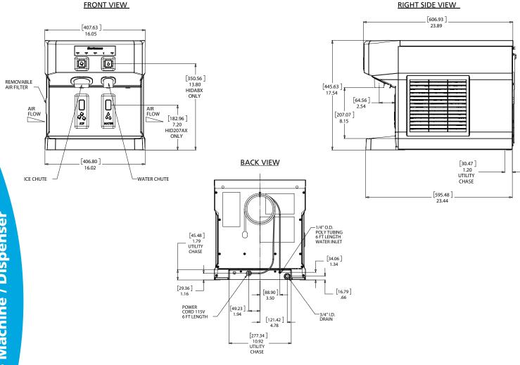
Installation Note: Allow 6" space at left, back and right side for ventilation and utility connections. All models include 6' power cord with NEMA 5-15P plug
