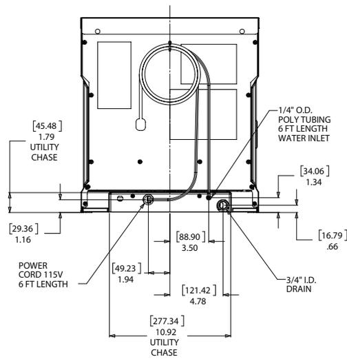
Installation Note: Allow 6" space at left, back and right side for ventilation and utility connections. All models include 6' power cord with NEMA 5-15P plug.
